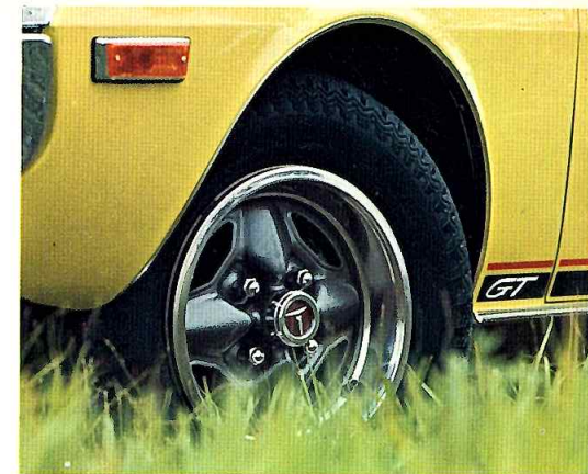
Special 185/70 HR 13 radial tires with wide wheel rims.
