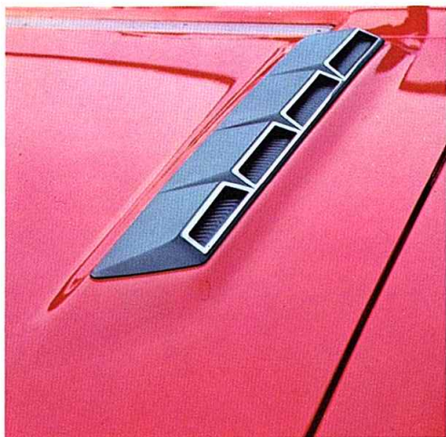
Hood louvers for better engine ventilation.
